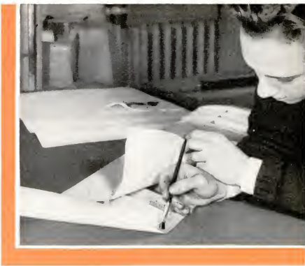
In covering the wing, start by cementing the paper to the center rib. Hold the paper in contact with pins as required
